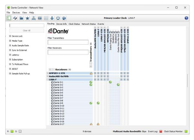
For talkover and priority, Dante channels will be picked automatically once the features are activated and the Dante channels are selected as input sources.
